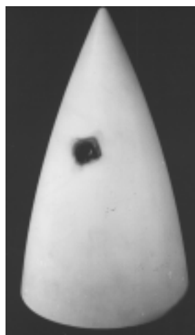
Fig. 4. Specimens from pyroceramic (1–3) and crystallized initial monolithic lithium aluminosilicate glass (4) with holes burned by an acetylene torch (specimen 4 has concentric through-thickness cracks).
